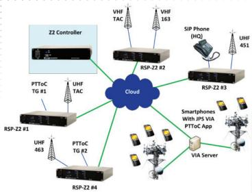
**Above**: Multiple RSP-Z2s, along with a single Z2 Controller unit, can be connected to create a wide area interoperability system with as many as 80 endpoints. This image shows a small system with eight different endpoints interfaced via four RSP-Z2s.
