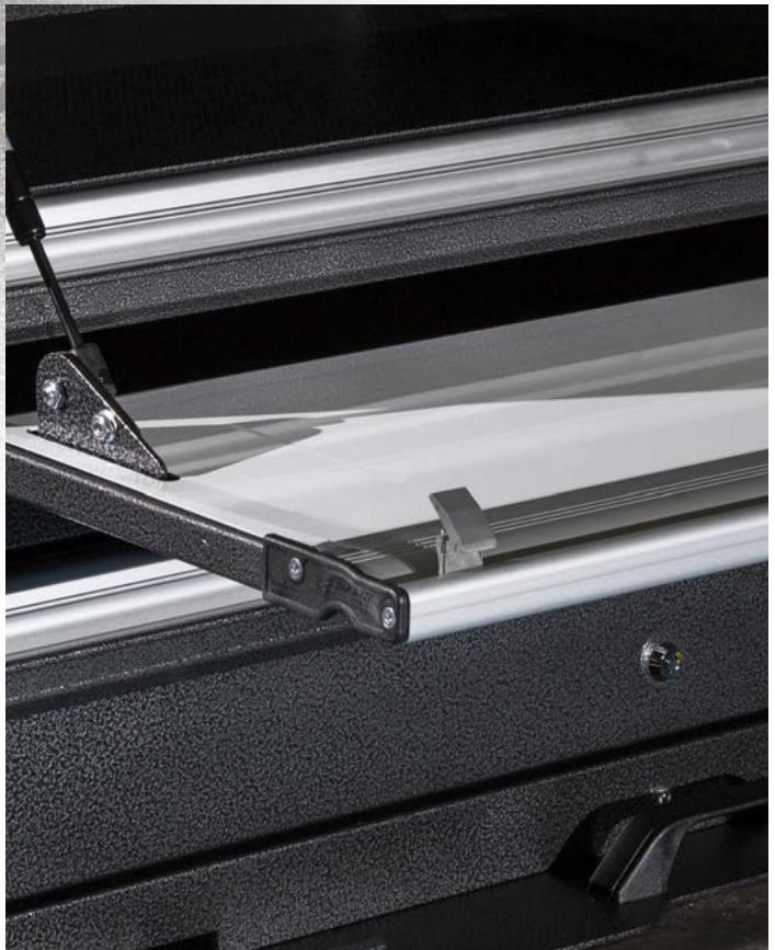
Dual composite latches stay closed
