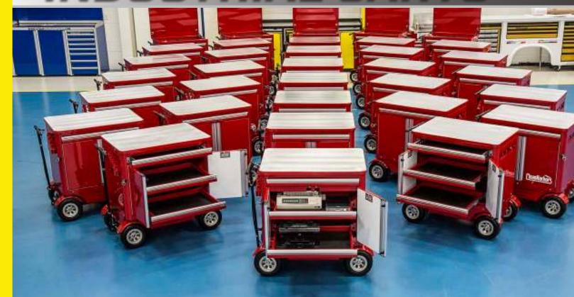
Mobile workstations built on the Hot Rod chassis. These carts are designed to the customers specifications for storage with electrical pre wired and MotionLatch $^{\text{TM}}$  adjustable shelves.
