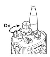
If the radio fails the self test, you hear a low-pitched tone and a numeric error code appears on the display. Turn off the radio, check the battery, and turn the radio on. If the radio fails the power-up test again, record the error code and contact your system administrator or an authorized radio technician.
