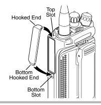
While holding the top end, swing the rounded end into place at the bottom of the connector. Press firmly until it snaps into place.
