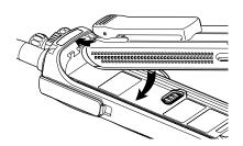
3 Push the battery down toward the radio until the battery clicks into place.
