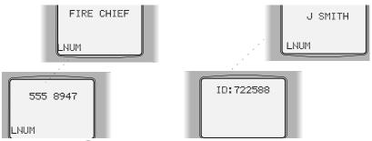
Note: Press — directly below the LNUM softkey to access the Last telephone NUMber dialed or the Last ID NUMber transmitted/received.
