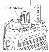
The LED lights up solid green while the radio is transmitting and blinks when the radio is receiving.
