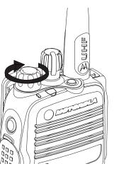
If your radio does not power up, check your battery. Make sure that it is charged and properly attached. If your radio still does not power up, contact your dealer.
