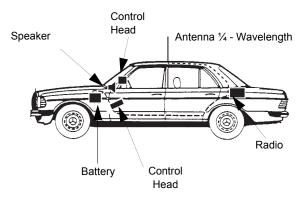
Figure 2-2 Typical Remote Mount Configurations
