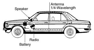
Figure 2-1 Typical Dash Mount Configuration
