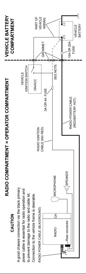
Figure 2-11 Cabling Interconnect Diagram for Dash Mount
