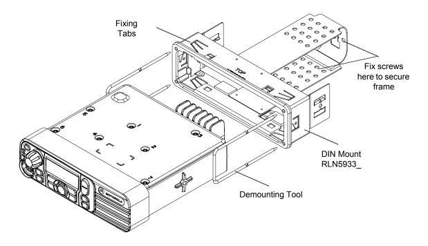
Figure 2-9 Dashboard Mounting for MOTOTRBO XPR 4000 Series
