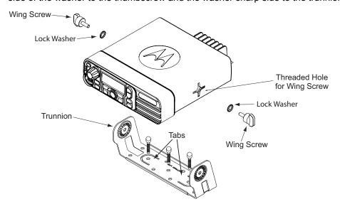
Figure 2-6 Transmission Hump Trunnion Mounting
