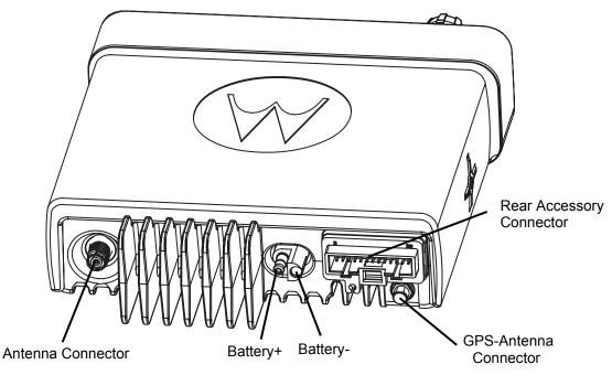
Figure 1-5 Back View of the Mobile Radio
