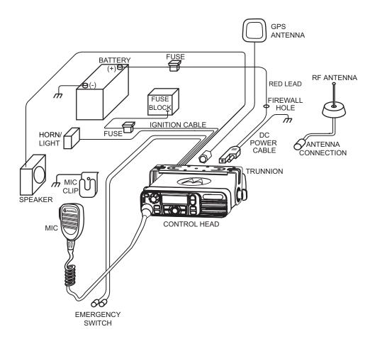
Figure 2-3 Radio Installation (Dash Mount)
