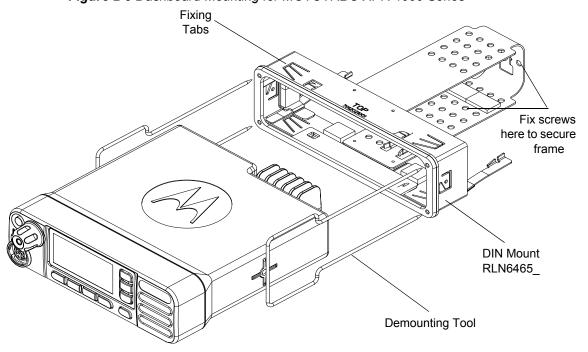
Figure 2-10 Dashboard Mounting for MOTOTRBO XPR 5000 Series
