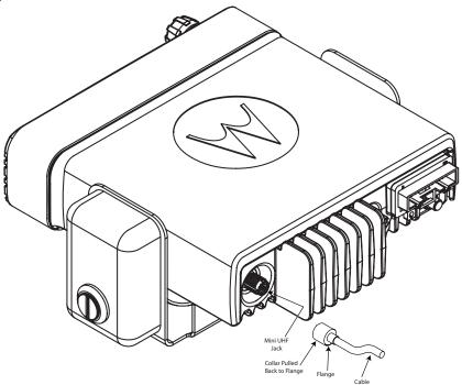
Figure 2-14 Mini-UHF Connection
