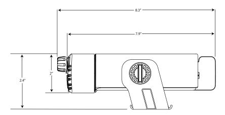
Figure 1-3 Side View of Dash Mount with Low Profile Trunnion for MOTOTRBO XPR 4000 Series
