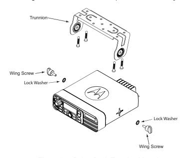
Figure 2-7 Below Dash Trunnion Mounting
