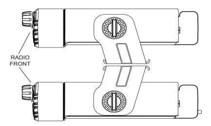
Figure 2-5 Trunnion Orientation for Above or Below Mobile
