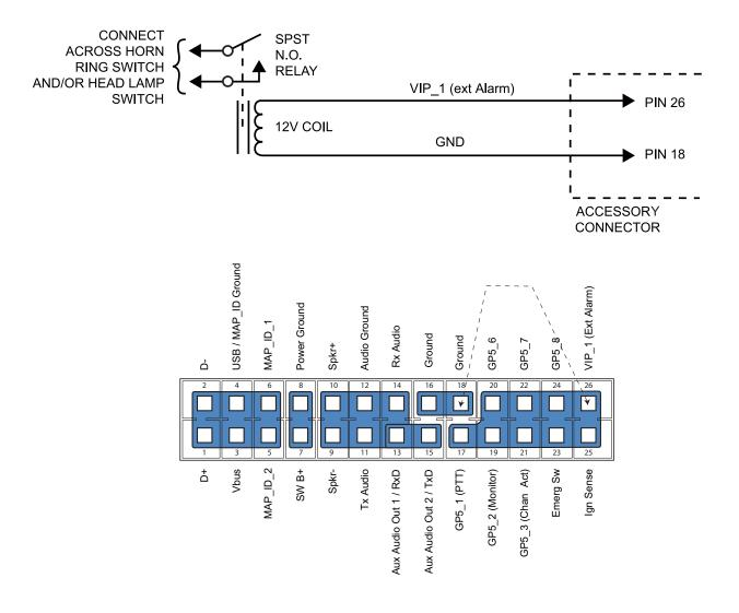
Figure 3-4 Horn and Lights Wiring Diagram
