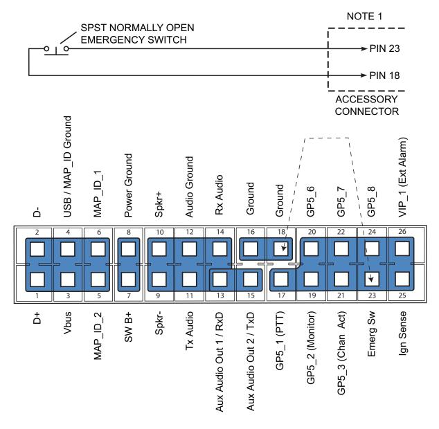
Figure 3-3 Emergency Switch Wiring Diagram
