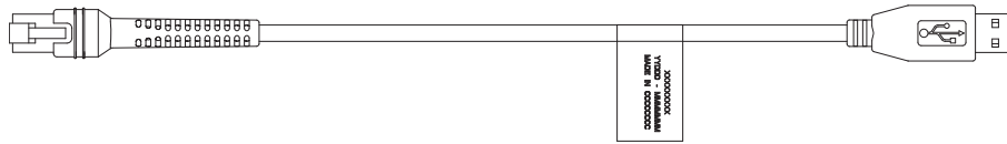
Figure 2-1 Front Telco MMP USB Programming Cable PMKN4147_
