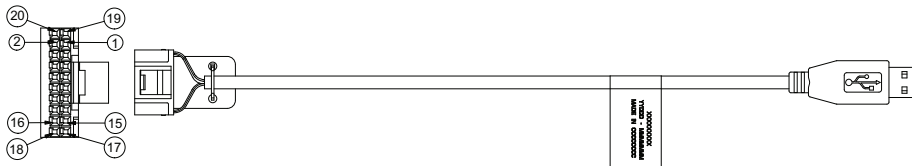
Figure 2-2 Back 20 Pin MAP USB Programming Cable PMKN4148_
