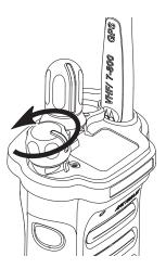
To turn off the radio, rotate the **On/Off/Volume Control Knob** counterclockwise until you hear a click.
