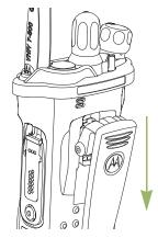
To remove the clip, use a flat-bladed object to press the belt clip tab away from the radio. Then, slide the clip downward and away from the radio.
