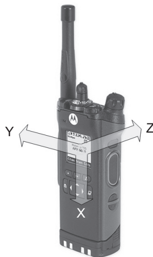
Figure 3-44. Directions of the Detectable Accelerations
