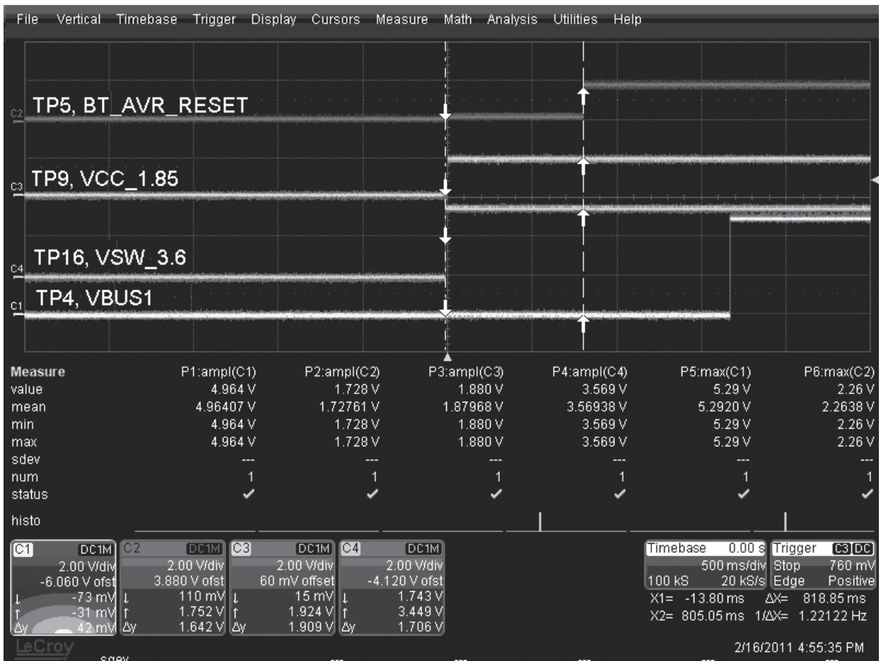
Figure 6-52. Startup – Timing Difference of TP5 to TP16 and Voltage Statistics
