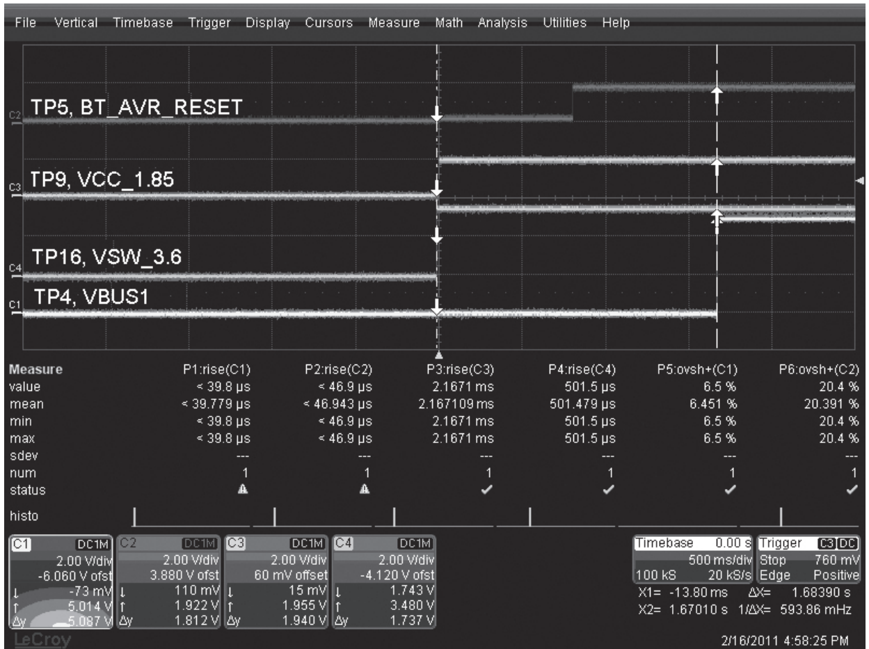
Figure 6-53. Startup – Timing Difference of TP4 to TP16 and Time Statistics
