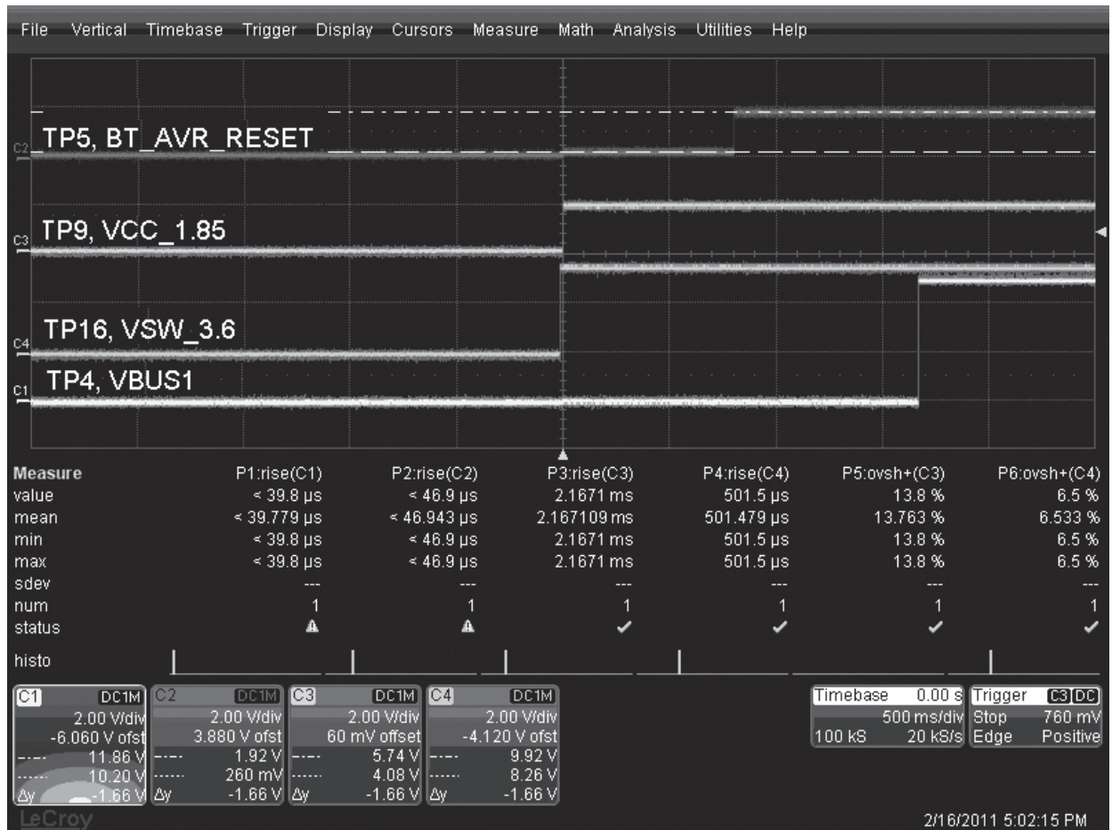
Figure 6-55. Startup – Vmax of TP5 and Time Statistics
