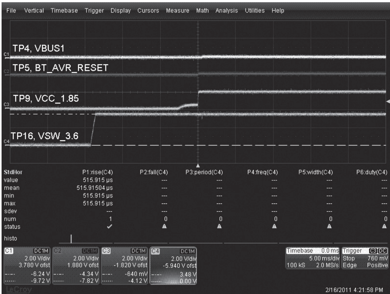
Figure 6-50. Startup Waveforms – Vmax of TP16
