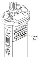
Your radio is designed to be submerged to a maximum depth of 6 feet, with a maximum submersion time of 2 hours. Exceeding either maximum limit may result in damage to the radio.
