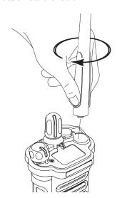
To remove the antenna, turn the antenna counterclockwise. Make sure you turn off the radio first.
