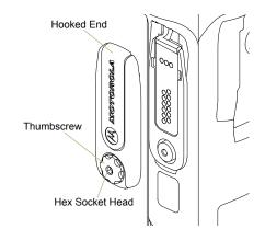
To remove the accessory connector cover, rotate the thumbscrew counterclockwise until it disengages from the radio. If the thumbscrew is too tight, use an Allen wrench to loosen it first.
