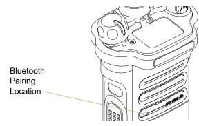
The range of Bluetooth operation is 10 meters line-of-sight communication. This is an **unobstructed** path between the location of the signal transmitter (your radio) and the location of the receiver (your device or accessory).
