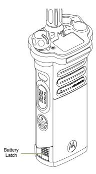
To remove the battery, turn the radio off. Squeeze the release latches at the bottom of the battery until the battery releases from the radio. Remove the battery from the radio.
