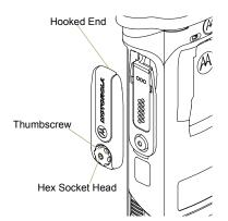
Rotate and lift the connector cover to disengage it from the radio.
