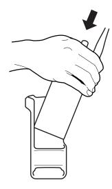
Position the radio within the carry holder with the main speaker facing outward. Slide the radio down into the carry holder until it clicks in place.
