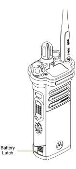
To remove the battery, turn the radio off. Squeeze the release latches on the bottom of the battery until the battery releases from the radio. Remove the battery from the radio.
