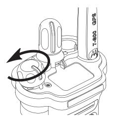
To turn off the radio, rotate the **On/Off/Volume Control Knob** counterclockwise until you hear a click.
