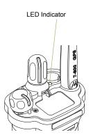
**Solid green** – Radio is powering up, or is on a non-priority channel while in the Scan List Programming mode.
