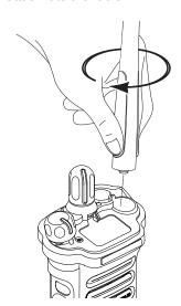
To remove the antenna, turn the antenna counterclockwise. Make sure you turn off the radio first.
