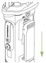
To remove the clip, use a flat-bladed object to press the belt clip tab away from the radio. Then, slide the clip downward and away from the radio.
