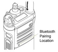
The range of Bluetooth operation is 10 meters line-of-sight communication. This is an **unobstructed** path between the location of the signal transmitter (your radio) and the location of the receiver (your device or accessory).
