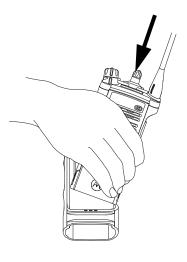
Position the radio within the carry holder with the main speaker facing outward. Slide the radio down into the carry holder until it clicks in place.
