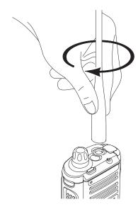
To remove the antenna, turn the antenna counterclockwise. Make sure you turn off the radio first.
