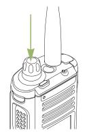
To turn off your radio, press and hold the MFK until the radio display shows *Power off?*, press the *Menu Select* button below *Yes* to power off.
