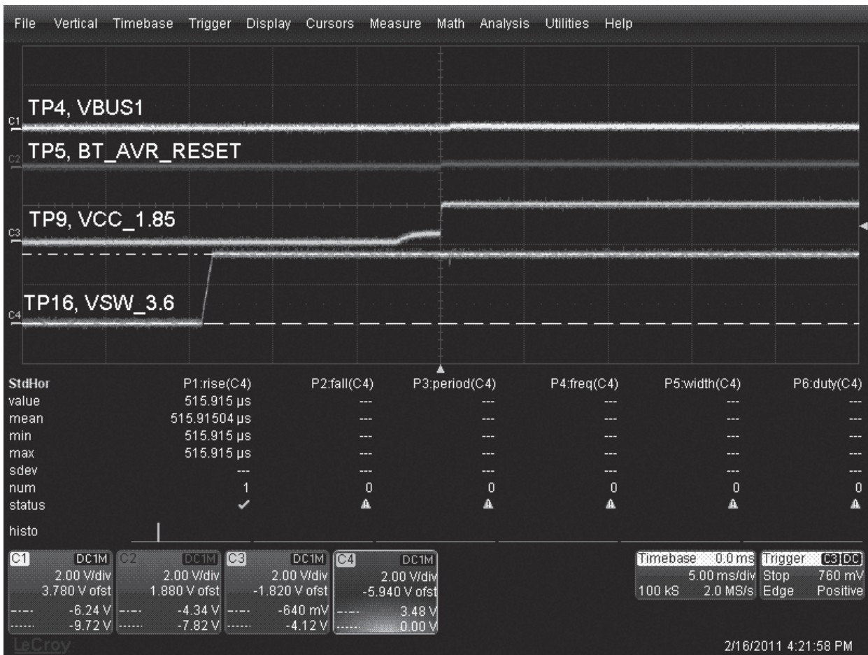
Figure 6-37. Startup Waveforms – Vmax of TP16
