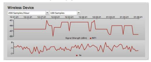
**Wireless Statistics:** View the signal strength and other wireless modem information. The wireless device's signal strength will only be displayed as long as it supports "Live Diagnostics." Sample rate and size can be adjusted from the dropdown boxes.
