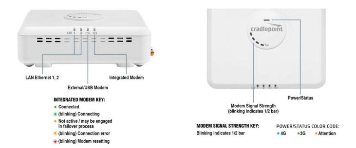
**Modem Signal Strength:** The bar LEDs indicate the signal strength from the active 3G/4G modem (Cradlepoint business-grade modem or USB modem). A blinking LED indicates ½ bar.
