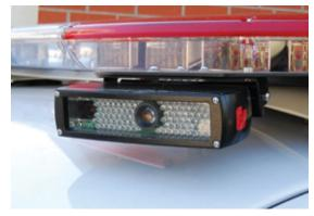
Motorola offers an ALPR Expansion Board for the MW810 that supports up to four Slate™ digital ALPR cameras from PIPS Technology, a Federal Signal Company. Working together, Motorola and PIPS have created an ALPR solution with unparalleled power, intelligence, and flexibility – and without the footprint of a separate ALPR processor.
