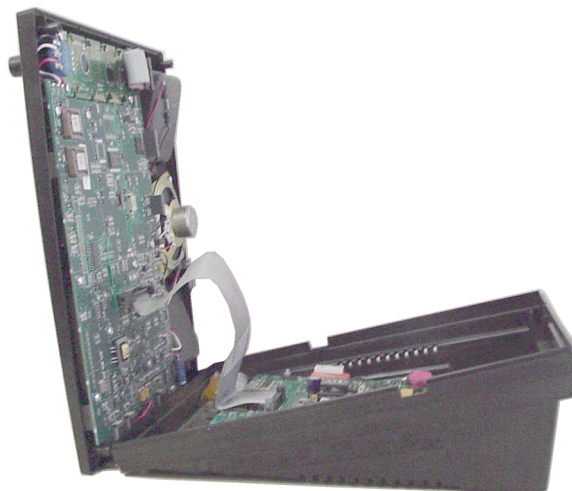
Figure 2-6: Separating Front from Rear Housing
